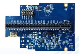
iWave's Gen4 x16 PCle FMC+ Module is designed to meet VITA 57.4 FMC+ standard.
