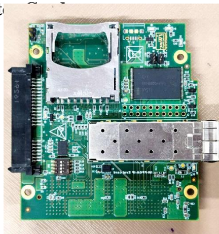
Figure 1: Test setup for SATA 3.0 Host Controller
