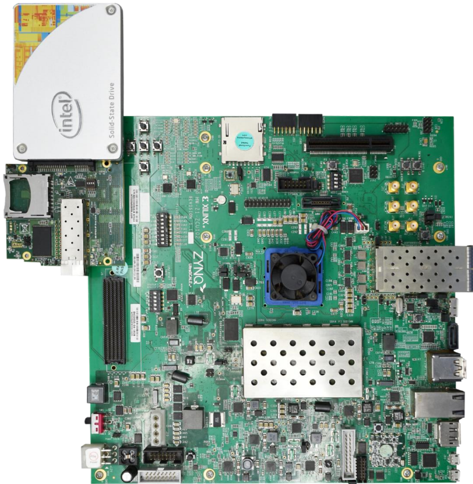
Figure 1: Test setup for SATA 3.0 Host Controller
