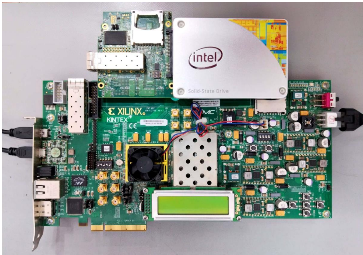
Figure 1: SATA 3.0 Host Controller setup
