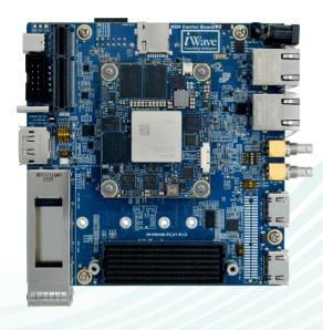
iWave's Versal Al Edge/Prime SoC development kit comprises of the Versal Al Edge/Prime SOM and REN Carrier board. The SOM is equipped with a 64-bit 4GB LPDDR4 RAM.
