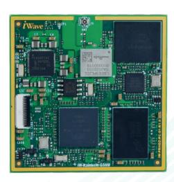
The i.MX 93 SoC based LGA Module is designed as per The Open Standard Module<sup>™</sup> specification (OSM). It integrates NXP's i.MX 93 offerings Dual Cortex A55 @ 1.7GHz, NPU with up to 0.5 TOP/s and IEEE 802.11 a/b/g/n/ac/ax Wi Fi + Bluetooth 5.3+ IEEE802.15.4 module.
