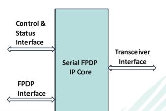
iW -sFPDP IP Core is based on ANSI/VITA 17.1-2015 Standards. This IP core provides a relatively simple protocol using maximum available data throughput with a minimum protocol for point-to-point data links. sFPDP links support a wide range of physical interfaces with the most common option being 10 gigabaud per second multimode fiber.
