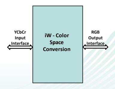
Color Space Converter converts video data from one color space format to another format. It is necessary to transfer data between devices which used different color space.
