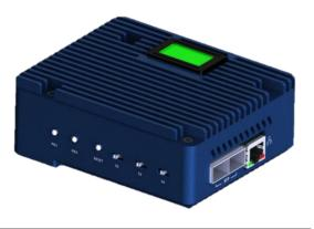
ARINC 818 DVR is a multi-channel record/playback system that accepts any form of ARINC818 video input with different resolution & refresh rate. The received ARINC818 video stream is encoded with the assist of an on-chip H.264/H.265 video codec engine which is capable of performing simultaneous compression and decompression of video streams and the encoded video is stored in SSD hard drive.
