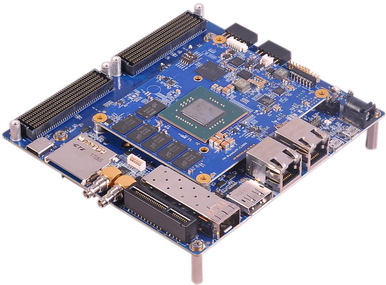
Figure 14: Zynq Ultrascale+ MPSoC SOM Development Platform
