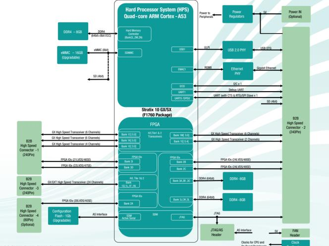
Compatible SoC: SX 2800 , SX 2500 , SX 2100 , SX 1650, SX 1100, SX850, GX 2800 GX 2500, GX 2100, GX 1650, GX 1100 and GX 850
