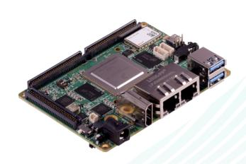
The i.MX8 Quad MAX/Quad Plus Pico ITX SBC integrates Dual Cortex A72 + Quad Cortex A53 Cores, Dual GPU systems,
