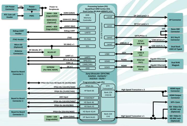
. CG devices supports Dual ARM Cortex-A53 & Dual ARM Cortex-R5. EG devices supports Quad ARM Cortex-A53. Dual ARM Cortex-R5 & Mali-400MP2 GPU. EV devices supports Quad ARM Cortex-A53, Dual ARM Cortex-R5 , Mali-400MP2 GPU & H.264/H.265 VCU.
