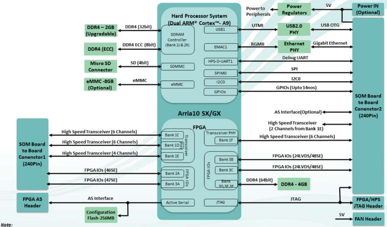
HPS (Hard Processing System) is supported only in Arria10 SoC family (SX) devices.
