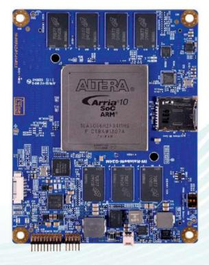
iWave's Arria 10 SoC System on Module is based on the Arria 10 SX family device with F34 package. The module is equipped with 32-bit DDR4 PS memory support for Hivith ECC and 64-bit DDR4 support for FPGA. All d the IOs and high speeransceiver blocks will be available on the SOM board to board connectors.
