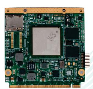
iWave's DM816x SOM is based on TI's DaVinci DM8168x ARM Cortex-A8+C674x DSP Microprocessor for faster and more robust applications. With extreme system and peripheral integration, the DSP+ARM MPUs provide multiple high-performance interfaces, such as PCle Gen2, HDMI 1.3, SATA2.0, Gigabit Ethernet and DDR3 interfaces.
