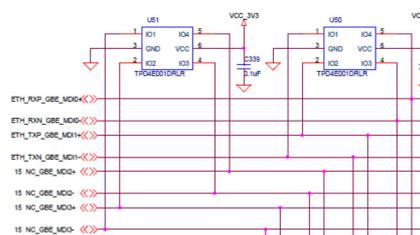
Another example for ESD protection in layout stage is shown below. For all externally accessible connectors chassis ground (earthing) are separately routed and low resistance current path to earth is provided for high current /voltage spikes.
